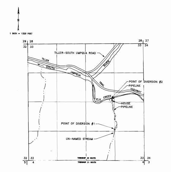
POINT OF DIVERSION #1 IS LOCATED 1270 FEET SOUTH AND 1340 FEET WEST FROM THE EAST 1/4 CORNER OF SECTION 33, BEING WITHIN THE NW 1/4 OF THE SE 1/4 OF SECTION 33. POINT OF DIVERSION #2 IS LOCATED 170 FEET NORTH AND 1450 FEET WEST FROM THE EAST 1/4 CORNER OF SECTION 33, BEING WITHIN THE SW 1/4 OF THE NE 1/4 OF SECTION 33, BOTH POINTS OF DIVERSION BEING WITHIN TOWNSHIP 30 SOUTH, RANGE 2 WEST, W.M., DOUGLAS COUNTY.
