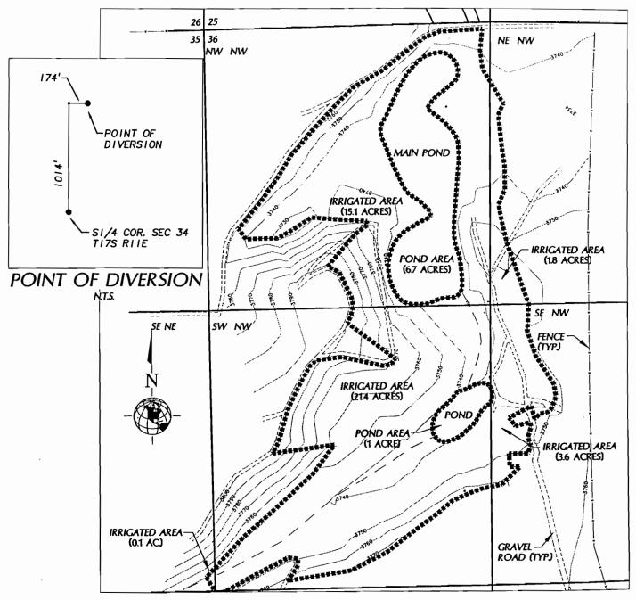
Note: The basis for this map is a 1994 topographic survey by W&H Pacific, notes from Thompson Irrigation for lands irrigated in 1994, and a field inspection on March 10, 1999. This map is for the purpose of locating a water right and has no intent to provide the location of property lines or legal dimensions.
