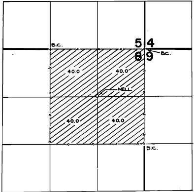
THE WELL IS LOCATED 1910 FT. 9. AND 1920 N. FROM THE N.E. CORNER OF SECTION 8.
