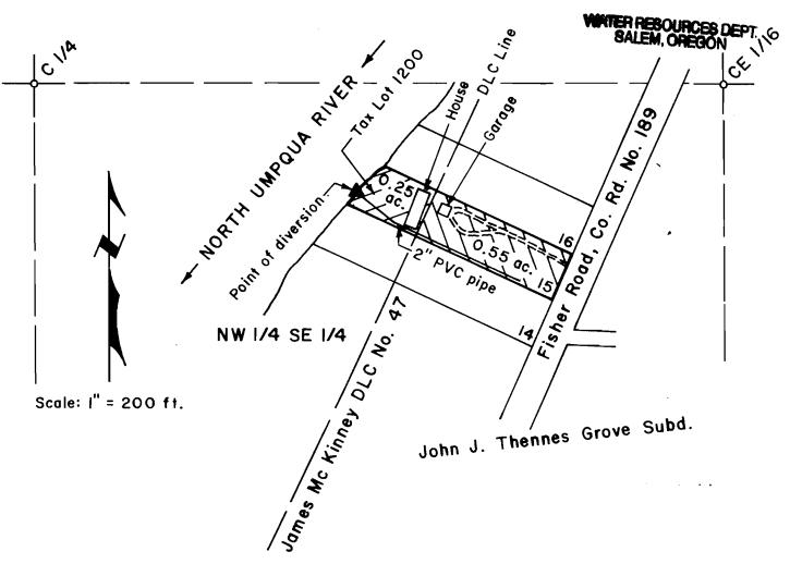
Point of diversion is South 200 ft. & East 600 ft. from the C1/4 corner of Section 27.
