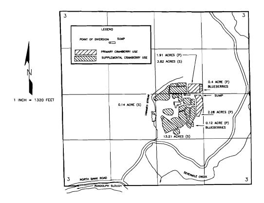
THE POINT OF DIVERSION IS LOCATED 2,365 FEET SOUTH AND 1,800 FEET WEST FROM THE NORTHEAST CORNER OF SECTION 3, BEING WITHIN THE NW% OF THE SE% OF SECTION 3, TOWNSHIP 28 SOUTH, RANGE 14 WEST, W.M., COOS COUNTY.
