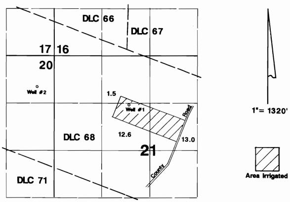
Well #1 located 1360'S & 2070'E from NW corner Section 21. Well #2 located 870'S & 460'W from NE corner Section 20.
