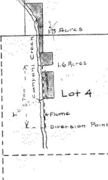
Note: Distance from SW corner Sec 35 to point of diversion was obtained by triangulation, bearing being determined by polar observation. Location of lot lines are only approximate.
