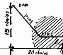
Pipe line to begin at a point which is 20 chains West and 15 chains North of  $\frac{1}{4}$  Cor. on the east line of Sec. 36., T 10 S, R 5 W, W.M.; thence S  $50^{\circ}$  E 15 chains, thence East to the East line of Sec. 36 (End of Pipe Line)
