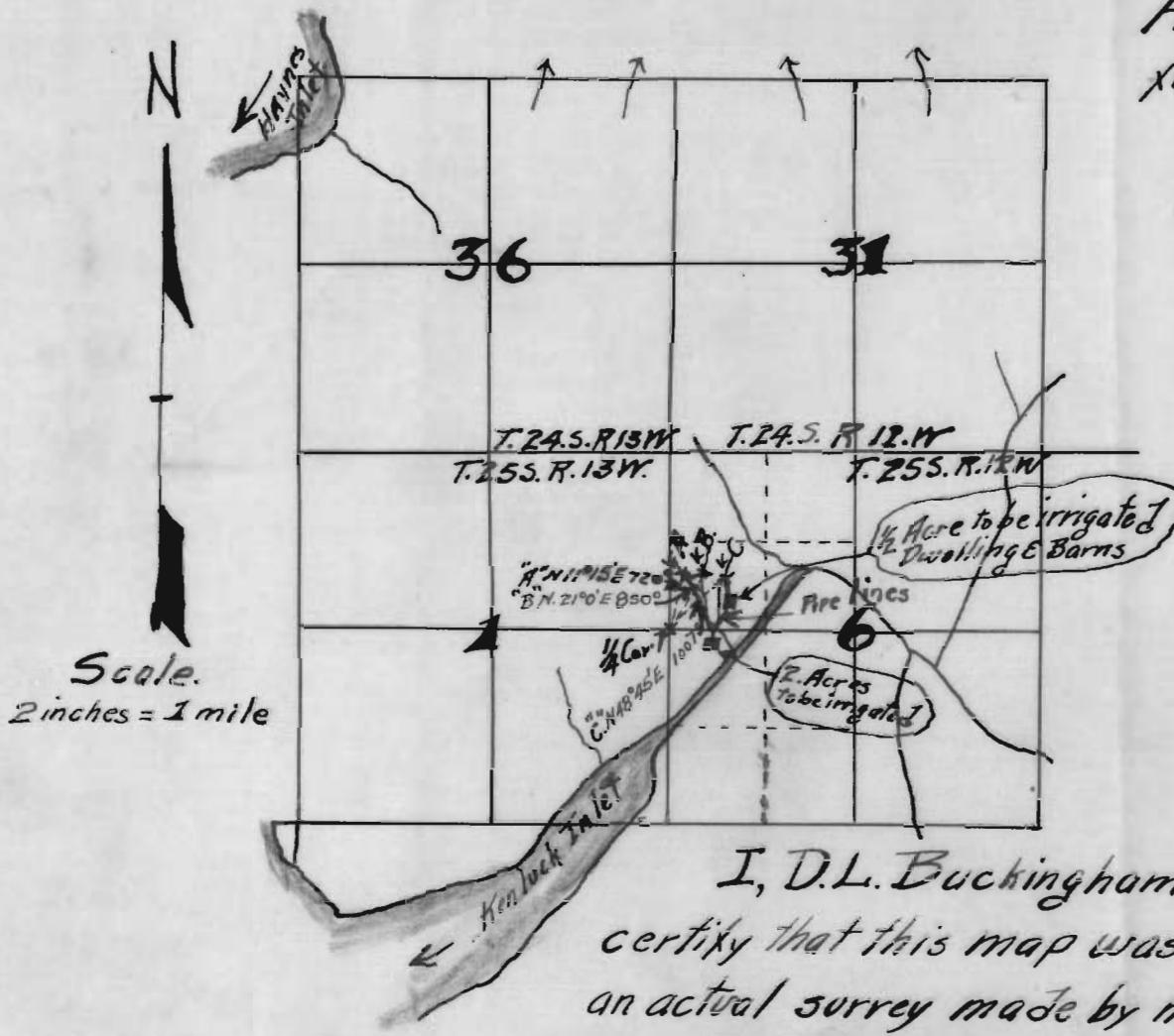
I, D.L. Buckingham, of Marshfield Ore., do hereby certify that this map was made from notes taken during an actual survey made by me Feb 8, 1927, and that it correctly represents the works described in the accompanying application, together with the location of the streams in the immediate vicinity.
