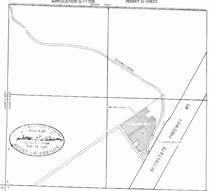
SUMP WELL #1 IS LOCATED 780 FEET NORTH AND 2100 FEET EAST FROM THE SOUTHWEST CORNER OF SECTION 6.
