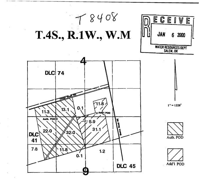
Auth. POD (well) is located 890'N & 2850'W from the SE corner of DLC 41. Add'l POD (well) is located 1200'N & 1100'W from the SE corner of DLC 41.
