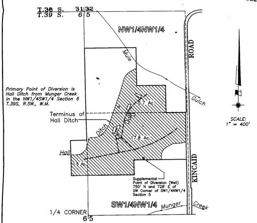
The ties to the well at the supplemental point of diversion are calculated from record data per Survey No. 374-77 in the Josephine County Surveyor's Office and measurements made to monuments found per said survey. The survey ties were made using a Wild T-1600 Theomat and a Distornat DI-1600 EDMI.
