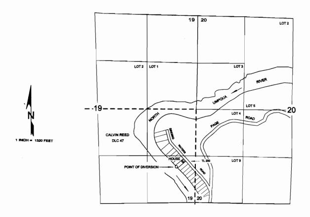
THE POINT OF DIVERSION IS LOCATED 1000 FEET NORTH AND 490 FEET WEST FROM THE SOUTHEAST CORNER OF SECTION 19, BEING WITHIN THE SE', SE', AS PROJECTED WITHIN CALVIN REED D.L.C. 47, OF SECTION 19, TOWNSHIP 26 SOUTH, RANGE 5 WEST, W.M.; DOUGLAS COUNTY.
