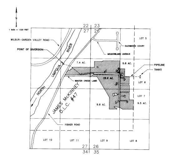
THE POINT OF DIVERSION IS LOCATED 1570 FEET SOUTH AND 1200 FEET WEST FROM THE NORTHEAST CORNER OF SECTION 27, BEING WITHIN THE SE 1/4 OF THE NE 1/4 OF SECTION 27, TOWNSHIP 26 SOUTH, RANGE 6 WEST, W.M., AS PROJECTED WITHIN THE JAMES MCKINNEY DONATION LAND CLAIM NUMBER 47, DOUGLAS COUNTY.
