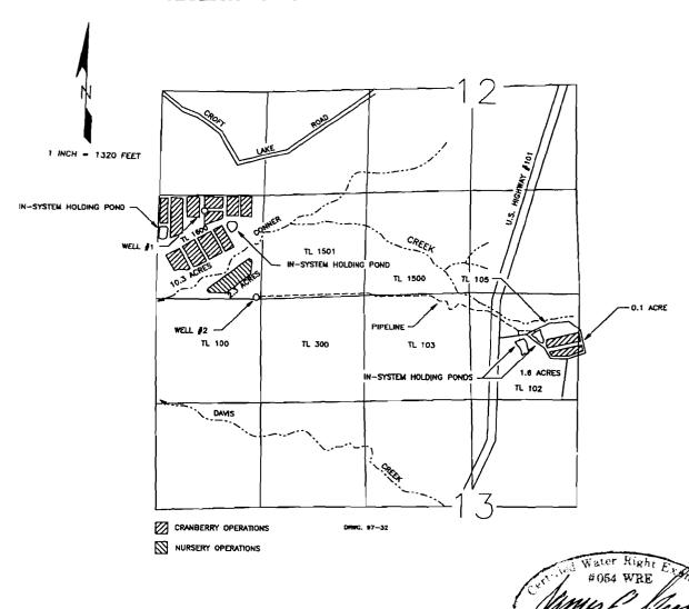
WELL # 1 IS LOCATED 1100 FEET NORTH AND 660 FEET WEST; WELL #2 IS LOCATED 5 FEET NORTH AND 20 FEET WEST, BOTH BEING FROM THE SOUTHEAST CORNER OF SECTION 11 AND BOTH BEING WITHIN THE SE1/4 SE1/4 OF SECTION 11, TOWNSHIP 30 SOUTH, RANGE 15 WEST, W.M., COOS COUNTY.
