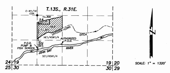
PROPOSED DIV. PT. IS 1820' S. AND 30' E. OF THE C-W1/16 COR. SEC. 19 AUTHORIZED DIV. PT. IS 1130' N. AND 40' W. OF THE S1/4 COR SEC. 19 - C-56303
