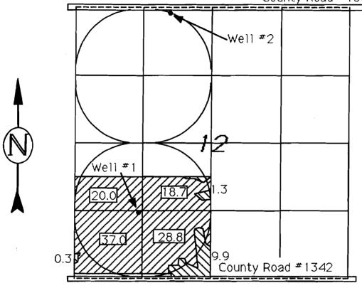
Well #1 Located 1280' North &1250' East of S.W. Corner of Section 12 Well #2 Located 135' South &1810' East of N.W. Corner of Section 12
