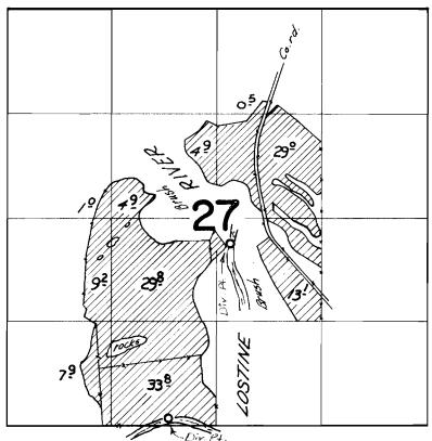
DIV. Pts. located 600 ft. W. \$ 100 ft. N. and 170 ft.E. \$ 2310 ft N. both from the 54 corner of Section 27
