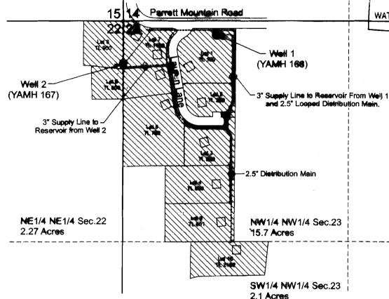
Well 1 (YAMH 168) is located 85 feet south and 550 feet east from the NW corner of Section 23. Well 2 (YAMH 167) is located 250 feet south from the NW corner of Section 23.
