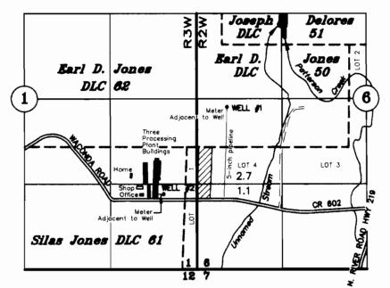
WELL #1: 620' N AND 620' E OF THE NE COR OF SILAS JONES DLC 61 WELL #2: 730' S AND 360' W OF THE NE COR OF SILAS JONES DLC 61
