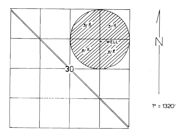
WELL 120' S. & 40' E. FROM THE CENTER OF THE NORTHEAST CORNER SEC. 30.
