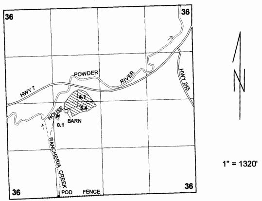
POD - 10 FEET NORTH AND 20 FEET EAST OF THE SOUTHWEST CORNER OF THE SE 1/4 SW 1/4 OF SECTION 36.
