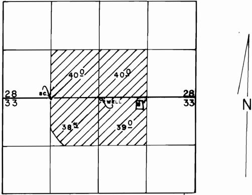
WELL LOC: 30'S & 1370'E FROM NW COR. OFNE 1/4 NW1/40FSEC 33.
