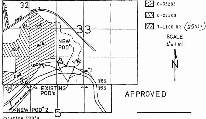
Existing POD's #1--858' N & 2970' W from SE cor. Sec.33 #2--660' N & 2464' W from SE cor. Sec.33 #3--1089' N & 3872' W from SE cor, Sec.33 #4--957' N & 4686' W from SE cor. Sec.33 all T8S, R25E, WM #5--1020' N & 2720' E from NW cor. Sec.5, T9S, R25E, WM.
