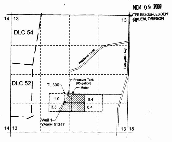
Well 1 (YAMH 51347) is located 1,370 feet north and 2,460 feet east from the SW corner of Section 13.
