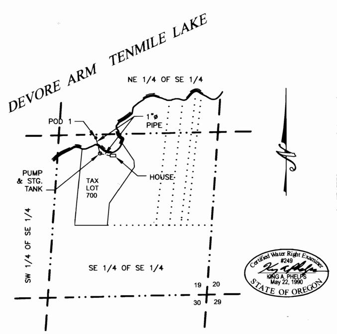
POINT OF DIVERSION (POD 1) IS 1,316' N AND 920' W OF THE SECTION CORNER COMMON TO 19, 20, 30 & 29.
