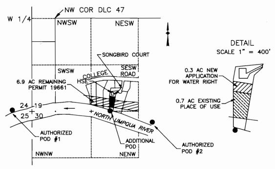
ADDITIONAL POD IS 2620 FT S AND 2180 FT E FROM W1/4 COR SEC 19 AUTHORIZED POD #1 IS 2600 FT S AND 550 FT W FROM W1/4 COR SEC 19 AUTHORIZED POD #2 IS 2940 FT S AND 3360 FT E FROM W1/4 COR SEC 19
