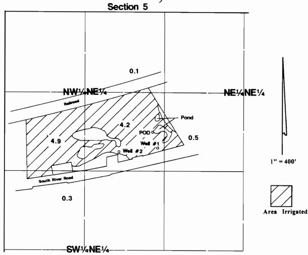
Well #1 is located 1140'S & 1260'E from the NW corner of NE1/4, Section 5. Well #2 is located 1170'S & 950'E from the NW corner of NE1/4 Section 5. POD is located 980'S & 1245'E from the NW corner of NE1/4 Section 5.
