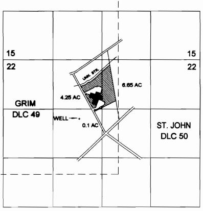
WELL LOCATED 1440 FT. N. & 5470 FT. E. FROM SW COR. GRIM DLC 49 WITHIN THE SEY, NWY, OF SECTION 22, AS PROJECTED WITHIN DLC 49
