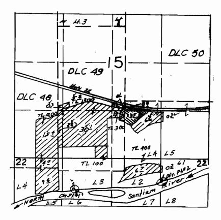
Diversion Point 1 is located 520 feet south and 400 feet east of the southwest comer of Stout DLC 49. Diversion Point 2 is located 250 feet south and 2770 feet east of the southwest comer of Stout DLC 49.
