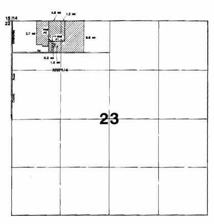
Well #1 located 610'S & 1020'E from NW corner Section 23. Well #2 located 604'S & 1014'E from NW corner Section 23.
