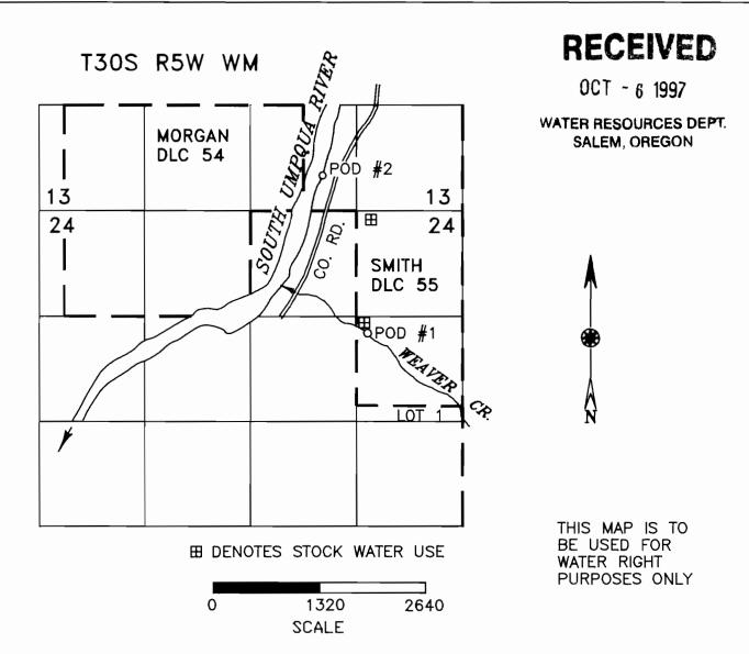
POD #1 IS 1530 FEET SOUTH AND 1180 FEET WEST FROM THE S.E. CORNER OF SECTION 13
