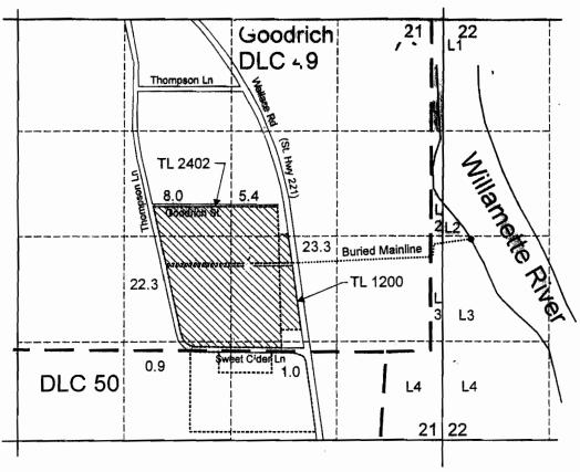
Diversion Point is located 1,440 feet north and 500 feet east from the SE corner of DLC 49.
