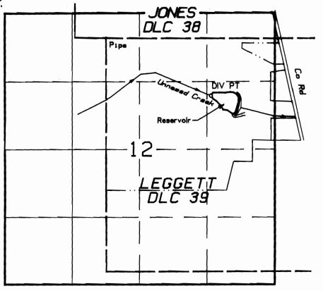
RESERVOIR DI'V PT SOUTH 1120' & EAST 2035' FROM NW CORNER DLC 39 DAM CENTERLINE SOUTH 1330' & EAST 2560' FROM NW CORNER DLC 39
