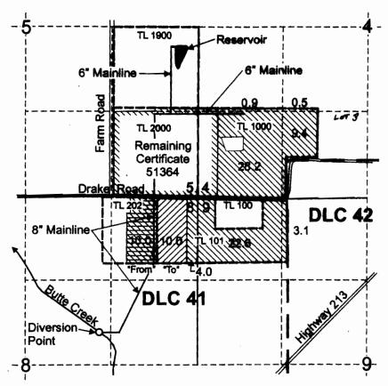
Point of Diversion is located 2,110 feet south and 1,120 feet east from the N 1/4 corner of Section 8.
