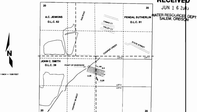
THE POINT OF DIVERSION IS LOCATED 2285 FEET NORTH AND 290 FEET WEST FROM THE SOUTH QUARTER CORNER OF SECTION 20; BEING WITHIN THE NE' SW' OF SECTION 20, AS PROJECTED WITHIN D.L.C. 39, TOWNSHIP 25 SOUTH, RANGE 5 WEST, W.M.; DOUGLAS COUNTY.
