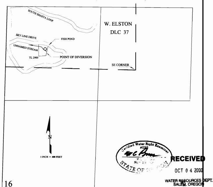
THE POINT OF DIVERSION IS LOCATED 295 FEET NORTH AND 1290 FEET WEST FROM THE SOUTHEAST CORNER OF W. ELSTON D.L.C. No. 37, BEING WITHIN THE NW'/SW'/4 OF SECTION 16, TOWNSHIP 18 SOUTH, RANGE 3 WEST, W.M.
