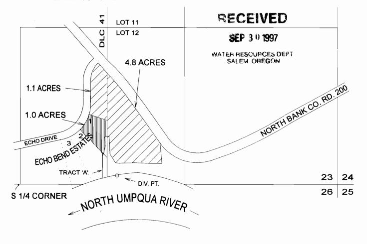
THE DIVERSION POINT IS LOCATED 72 FEET NORTH AND 810 FEET EAST FROM THE SOUTH 1/4 CORNER OF SEC. 23, T 26 S, R 5 W, W M, BEING WITHIN THE SW 1/4 OF THE SE 1/4 OF SEC. 23 (GOV'T LOT 12).
