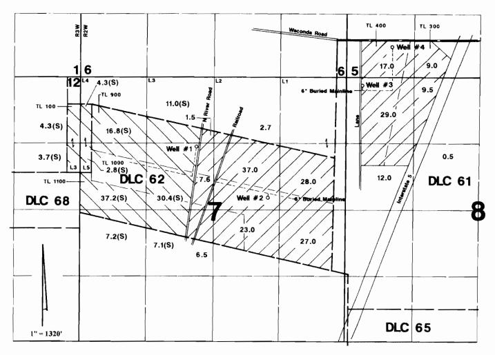
Well # 1 is located 1260'N & 330'W; Well # 2 is located 230'N & 1100'E;— both from the center of Section 7. Well # 3 is located 160'S & 300'E; Well # 4 is located 600'N & 890'E;— both from the NW corner of Section 8.
