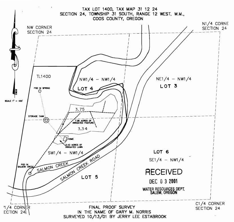
P.O.D. IN SPRING BEARS N14"21'15"E 1711' FROM THE W1/4 CORNER OF SECTION 24. P.O.D. IN SALMON CREEK BEARS N32'14'25"E 533' FROM THE W1/4 CORNER OF SECTION 24.
