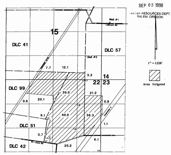
Well #1 is located 480'N & 2550'W from the center of Section 14. Well #2 is located 890'N & 20'E from SE corner of DLC 41.
