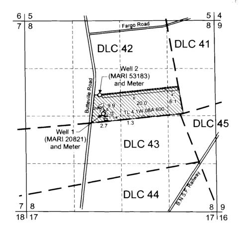
Well 1 (MARI 20821) is located 70 feet north and 2,130 feet east from the W 1/4 corner, Section 8. Well 2 (MARI 53183) is located 590 feet north and 2,030 feet east from the W 1/4 corner, Section 8.
