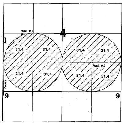
Well #1 located 80'S & 815'E from W1/4 corner of Section 4. Well #2 located 1330'S & 4018'E from W1/4 corner of Section 4.
