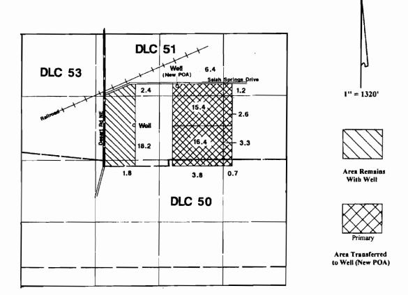
Well is located 860'N & 620'E from SW corner of T. Shaw DLC 51.
