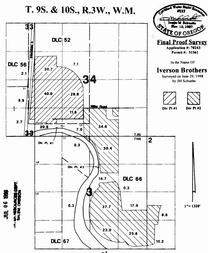
Div. Pt. #1 is located 450'N & 1020'E from SE corner Section 34. Div. Pt. #2 is located 1520'S & 3010'E from NW corner Section 3.
