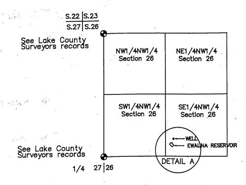
The center of Ewauna Reservoir is located S.31°21'52"E., 2750.46 ft., from the NW section corner of section 26. The measurement is from GPS survey by Peter A. Olson in 1999. The bearings are based on GLO record bearing of N.0°04"W., for the north half of the west line of section 26, as shown on the official survey approved June 1, 1935. The water stored in this reservoir is to be used for fire suppression activities, maintenance of Forest Service roads and stock watering.
