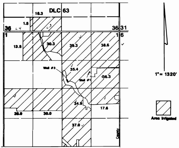
Well #1 located 1860'S & 1370'W from NE corner Section 1. Well #3 located 2280'S & 2300'W from NE corner Section 1.
