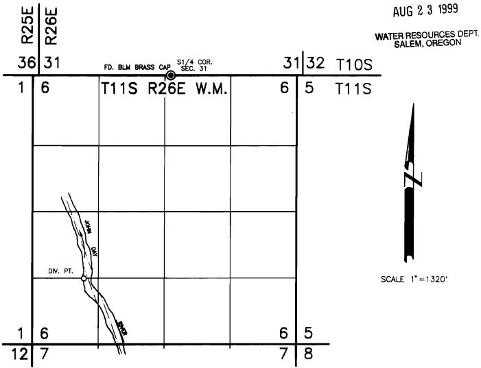
Diversion Point is 4050' S. and 1610' W. of the S1/4 Cor. Sec. 31, T.10S., R.26E.
