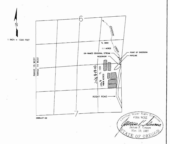
THE POINT OF DIVERSION IS LOCATED 220 FEET NORTH AND 50 FEET WEST FROM THE SOUTHEAST CORNER OF SECTION 6; BEING WITHIN THE SE1/4 SE1/4 OF SECTION 6, TOWNSHIP 29 SOUTH, RANGE 14 WEST, W.M., COOS COUNTY.
