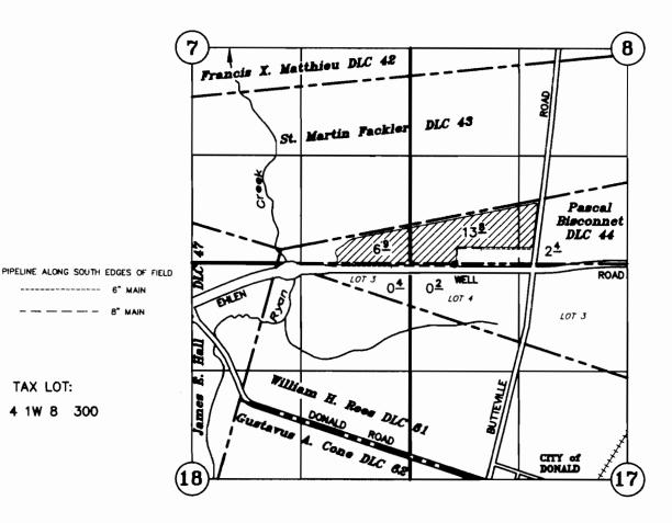
WELL: 174' S AND 2108' E OF THE NW COR OF BISCONNET DLC 44 ELECTRICAL METER 8'S AND 4' W OF WELL
